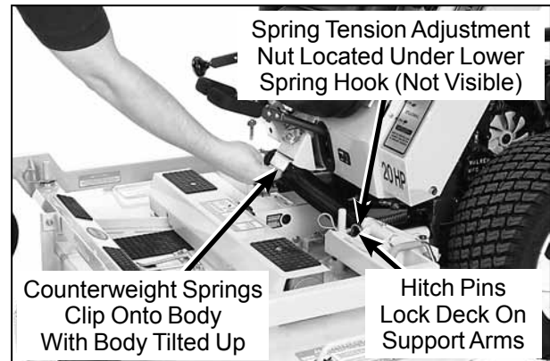
Deck Counterweight Spring Installation
