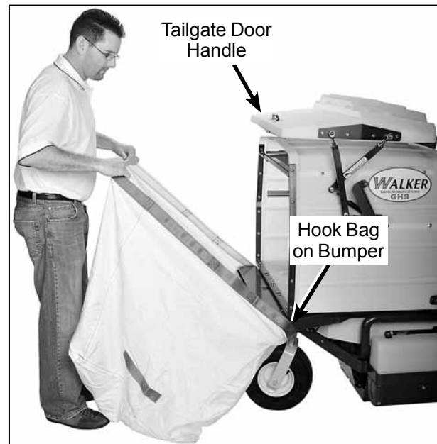
Positioning Dump Bag on Catcher
