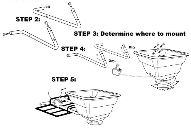
**STEP 3:** Determine whether to mount on the front or the back luggage rack. Depending on whether the M20 is mounted to the front or rear rack, you will need to install (#4) Control assembly to either the right (#11) or left (#15) Frame tube to allow for use with the non-throttle hand. Wait until the unit is mounted to the Quad before installing the Control.
