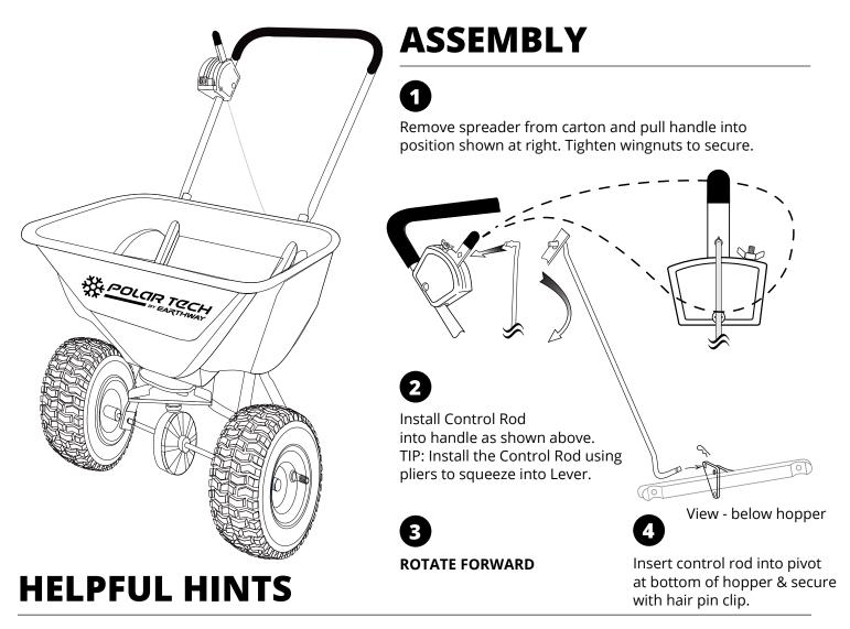
Your spreader is almost ready to use. Attaching the control rod and unfolding the handle will require a pair of pliers to insert pins to secure the control rod. **NOTE: The large opening is designed to allow ice melt to flow through spreader without the need for an agitator. Prior designs utilized an agitator, this model does not.**
