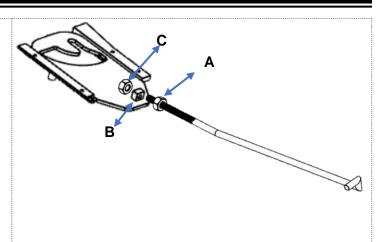
**Step 11:** Install handle shaft to lower handles and pivot & bracket assembly as shown. Using ¼-20 x 2" bolts and locknuts. **TIGHTEN BOLTS AND NUTS NOW**.
