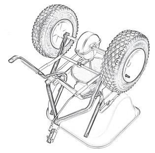
**3.** Ensure that the axle bearings are pushed into the axle bushing on both sides as shown. Install drive wheel (both wheels are interchangeable) to axle using pin hole nearest to
