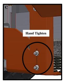
5. Attach Rear Light Bracket to Fender and Fertilizer Box Platform with two  $5/16 \times 1$  bolts and two 5/16 nuts from step 1.
