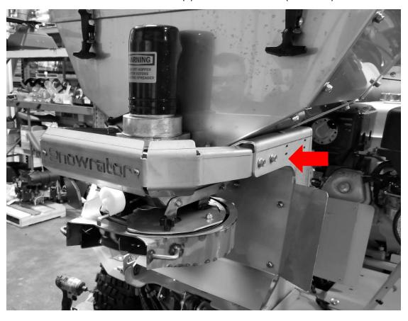
ROTATE SHAFT TO GAIN ACCESS TO BOTTOM SET SCREW IN COLLAR. LOOSEN ONLY, DO NOT REMOVE COMPLETELY.
