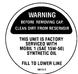
Hydrostat Oil Reservoir (5810-2)
