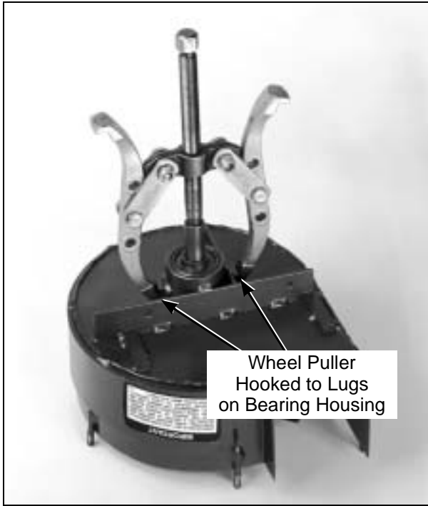
Pressing Blower Wheel Out of Housing
