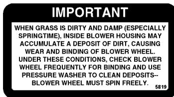
Top of Blower Housing (5819)
