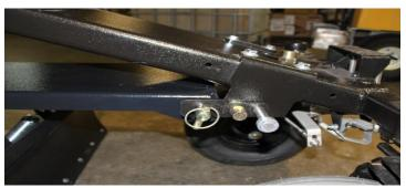
(Snow Blade locked into the Aerator Front Frame)
