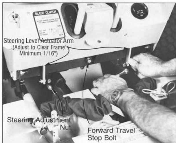
PHOTO 5-16 Forward Speed Control Stop and Steering Lever Adjustment
