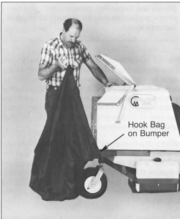
PHOTO 4-6 Positioning Dump Bag on 6.7 Bushel Catcher
