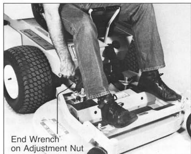
PHOTO 5-18 Adjust Transmissions for Straight Travel
