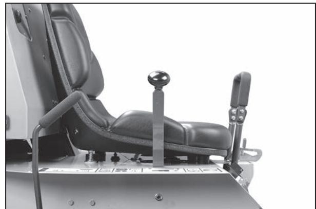
Correct FSC Lever NEUTRAL-PARK Position
