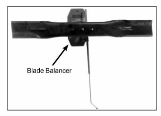
**Blade Balanced on Magnetic Wall-Mounted Balancer**
