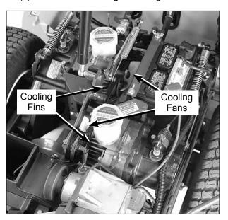
**Hydrostatic Transmission Cooling Fins**
