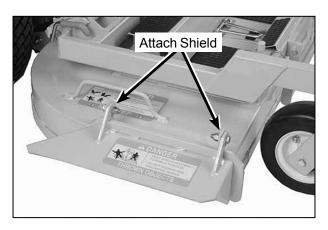
Discharge Shield Installation on Side Discharge Deck
