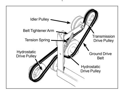
**Ground Drive Belt Assembly (Engaged)**
