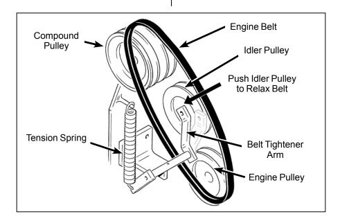
**Engine Belt (Disengaged)**
