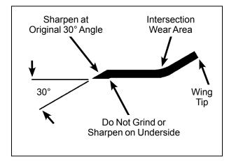
**Mower Blade Profile For Sharpening**
