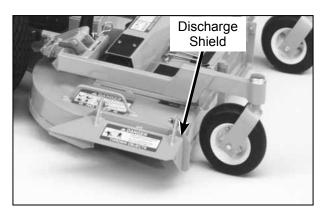
Side Discharge Deflector Shield in Lowest Position
