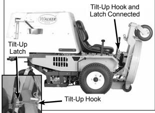
**Deck Secured in TILT-UP Position**
