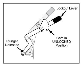
**Lockout Lever - Normal Operating Position**
