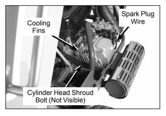
**Inspect and Clean Cylinder Head Cooling Fins** (Viewed from Left Side of Tractor)
