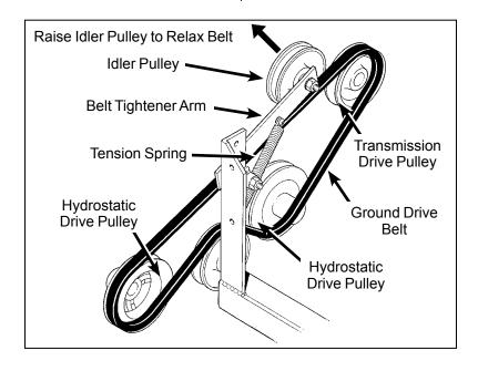
**Ground Drive Belt Assembly (Disengaged)**
