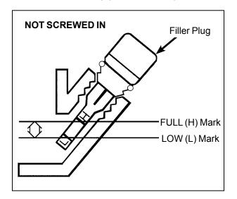
Dipstick Position for Checking Oil Level
