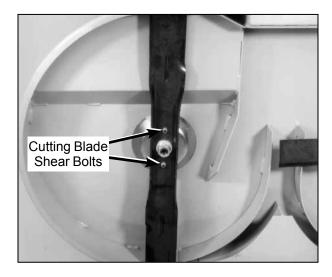
**Cutting Blade Shear Bolts**
