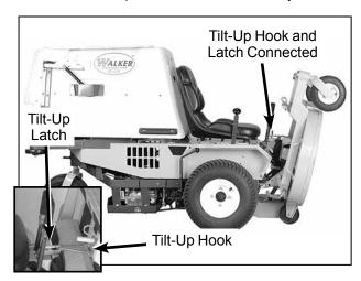
**Deck Secured in TILT-UP Position**
