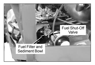
Fuel Filter and Fuel Shut-off Valve Location
