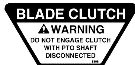
On Body Adjacent to Clutch Control Lever (5806)
