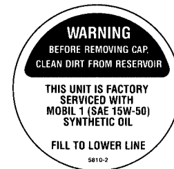
Hydrostat Oil Reservoir (5810-2)
