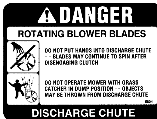
Adjacent to Blower Discharge Chute Through Body (5804)
