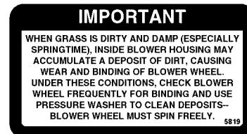
Top of Blower Housing (5819)
