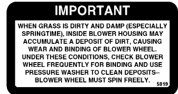
Top of Blower Housing (5819)
