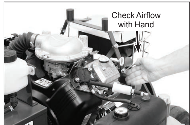
Cooling System Airflow
