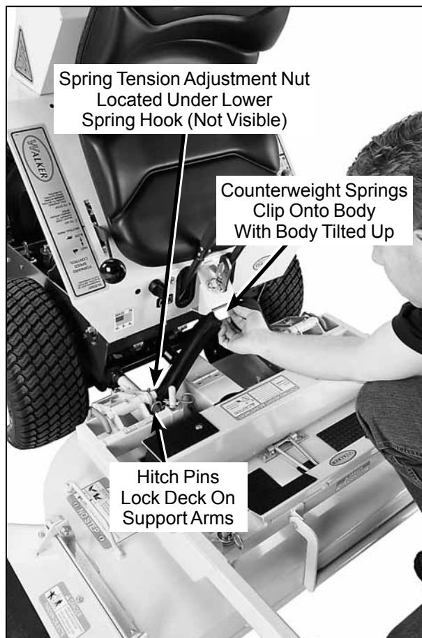
Deck Counterweight Spring Installation
