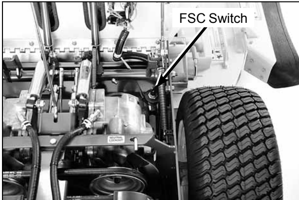
FSC Switch Location
