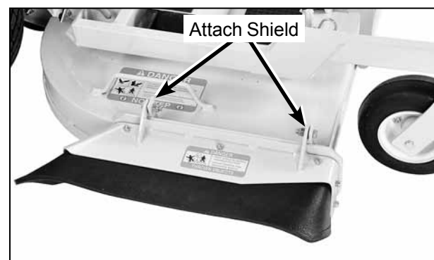
Deck Discharge Shield Installation
